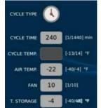
During a Time Cycle (clock icon in the *CYCLE TYPE* tab) the unit will run the cycle pulling down and holding the temperature inside the cavity at the desired temperature set in the "*AIR TEMP*." tab, for the desired target time set in the "*CYCLE TIME*" tab.
