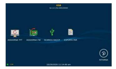
From the USB menu it's possible to upload the touch screen as well as the PCB software, download the HACCP records and export the parameters file.
