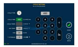
By factory default, the AIR TEMP. is -40°C, the fan speed is 10 and the storage temperature is -40°C.
