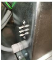
These units are equipped with a remote alarm plug for the connection to a remote alarm network.
