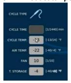
During a Temperature cycle (Needle probe icon in the *CYCLE TYPE* tab), the multi-core needle probes of the unit must be inserted inside a simulation bag. The Unit will run the cycle pulling down and holding the temperature inside the cavity at the desired temperature set in the "*AIR TEMP*." tab until the 4 cores of the needle probe reads the target temperature set in the "*CYCLE TEMP*." tab.
